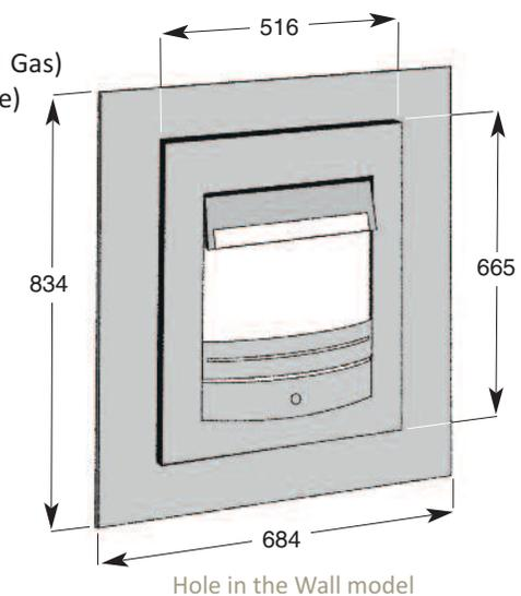
Measurements of visible parts only are shown. For further measurements or for fireplace model see page 27.
