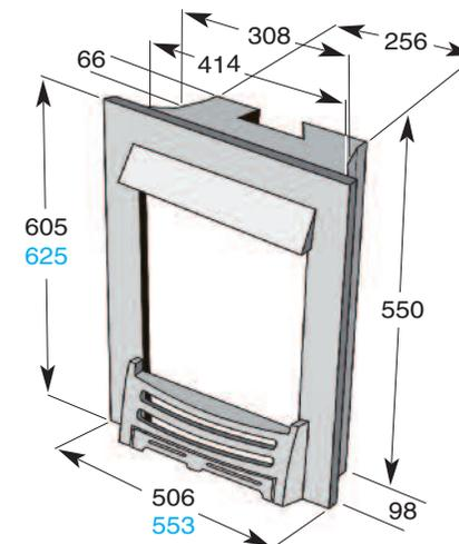
The Veo CF Slimline Royale is compatible with most Class 1 and Class 2 flues and almost all precast flues. The versatility of this fire is further enhanced by its being available for use with either Natural Gas or Propane.
