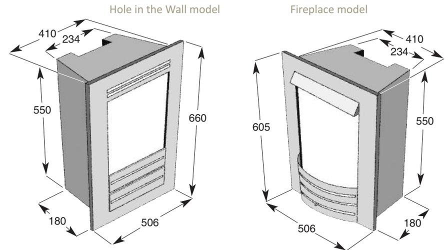
Vitesse CF Hole in the Wall model with Two-Tone Modern louvred Trim and Marfil Outer Frame
