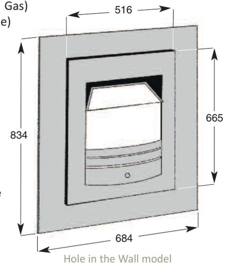
Measurements of visible parts only are shown. For further measurements or for fireplace model see page 35.
