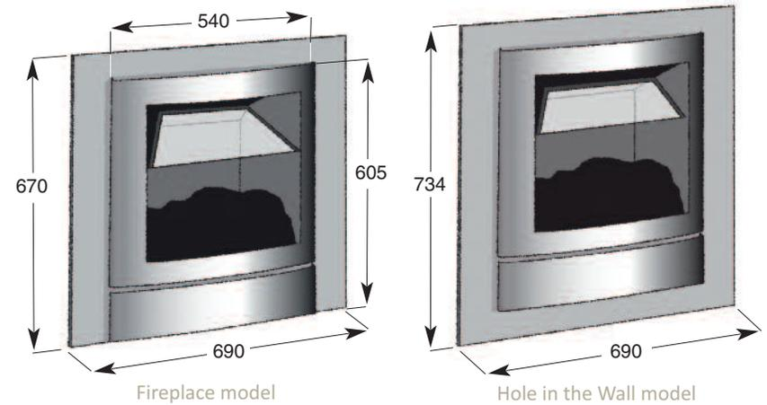
Measurements of visible parts only are shown. For further measurements please see page 31.
