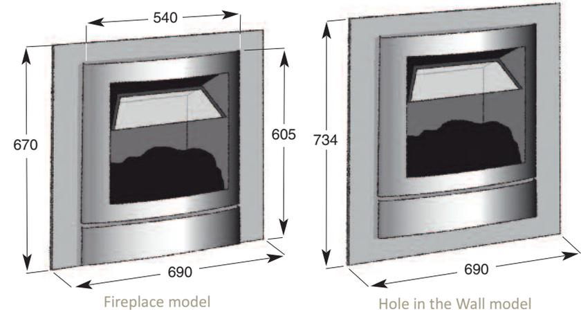
Measurements of visible parts only are shown. For further measurements please see page 35.
